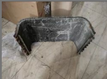
Window Ac Cooling Coil
